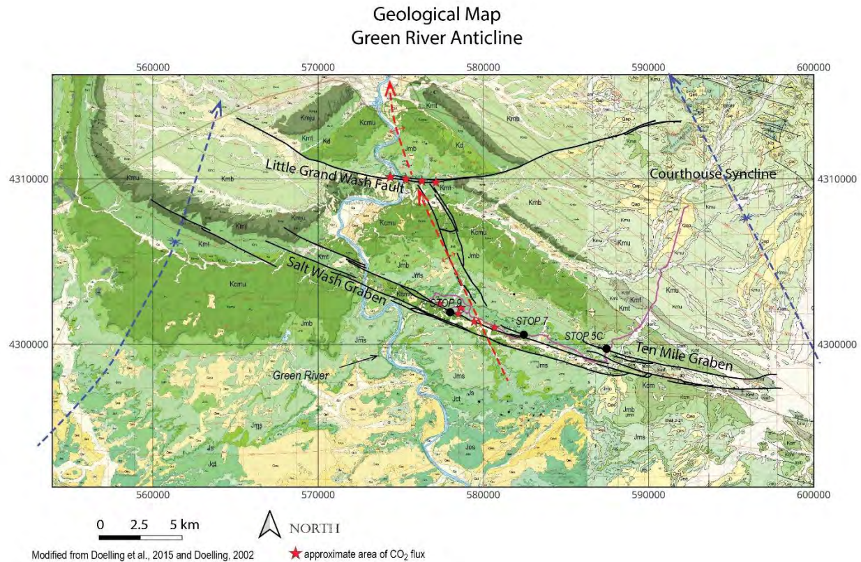
Figure 3. Geological map of the faulted Green River anticline with the principal faults highlighted and the main structures labelled. Modified from Doelling et al, 2015 and Doelling (2002).
